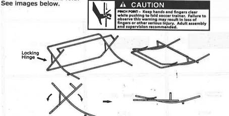
Note: Netting was removed to illustrate folding feature. The netting can remain on the product when folding for storage.
