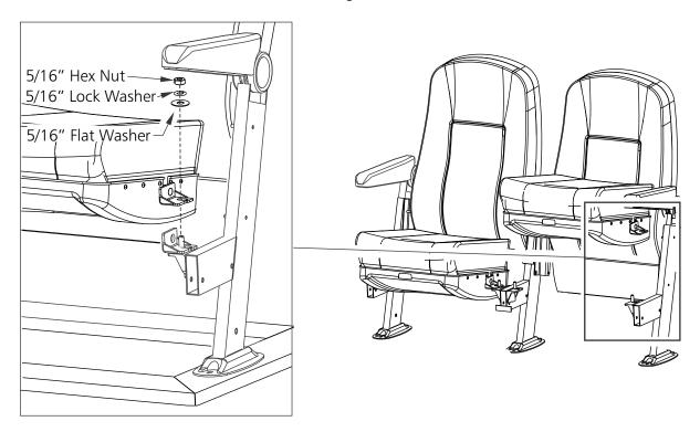
6. Attach center pad to seat frames as shown.
