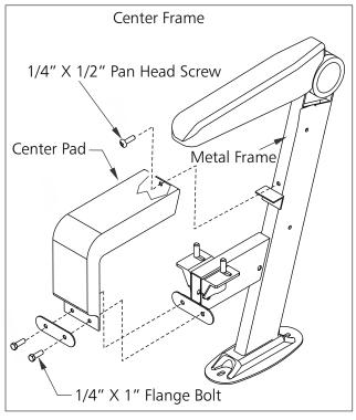
4. Seat backs can be attached at 2 angles. At the top of seat back bracket, use one of the holes to get the desired back angle and attach seat backs to metal fames as shown.
